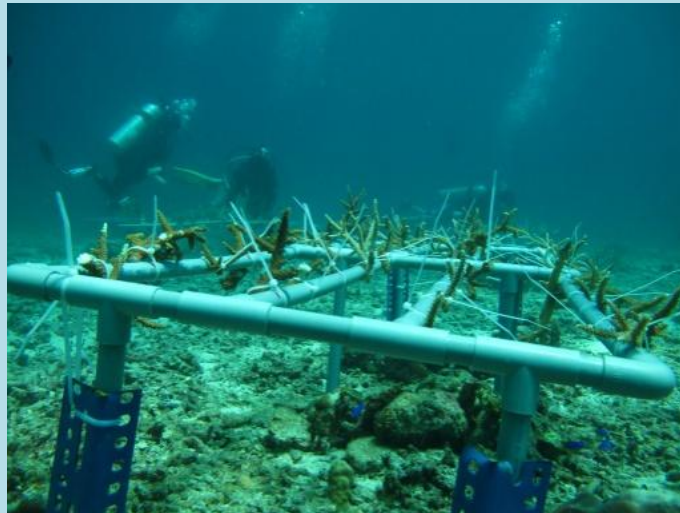
Figure 9: New frame design with legs integrated into the frame
