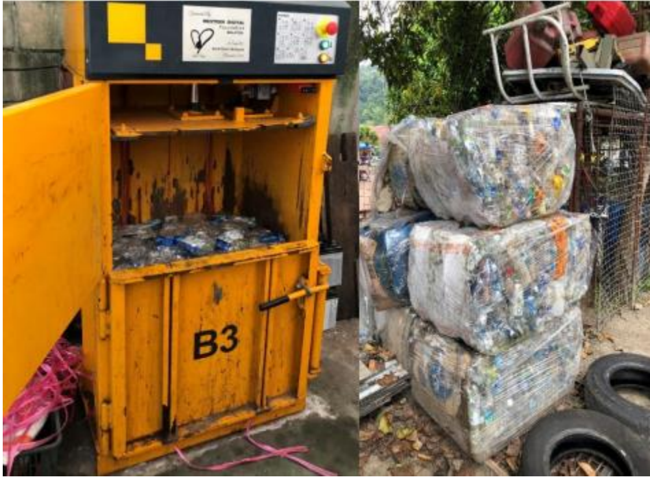
Baler machine on Tioman island (left) and the compressed plastic bottles (right) (Reef Check Malaysia)
