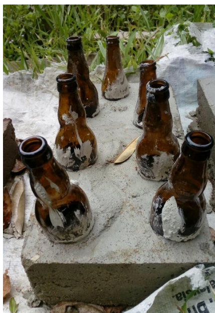
Figure 23: Cement block with old glass bottles
